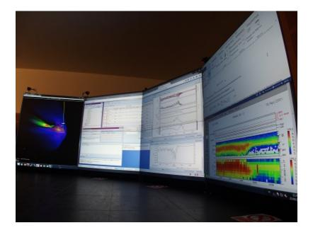
It is made up of 8 BARCO OLS-721 Full HD 70" modules equipped with overhead projectors. Real-time graphics rendering is possible thanks to a cluster of PCs equipped with NVIDIA K5000 graphics cards.
