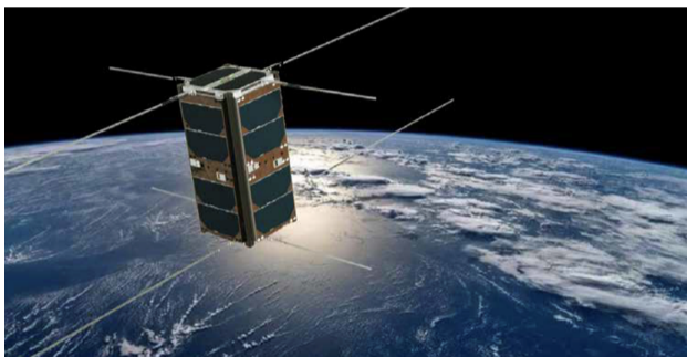
(b) Inspire-Sat 5 (Uvsq-Sat) spacecraft dedicated to Earth Radiation Budget (ERB) observations.
