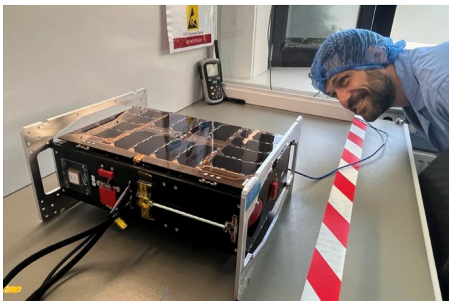
Figure 8: Inspire-Sat X (Uvsg-Sat NG) during integration in October 2023.
